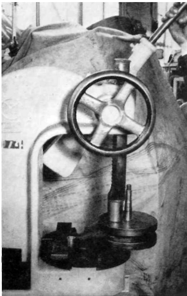
FIG. 27 Arbour Press for Flywheels
