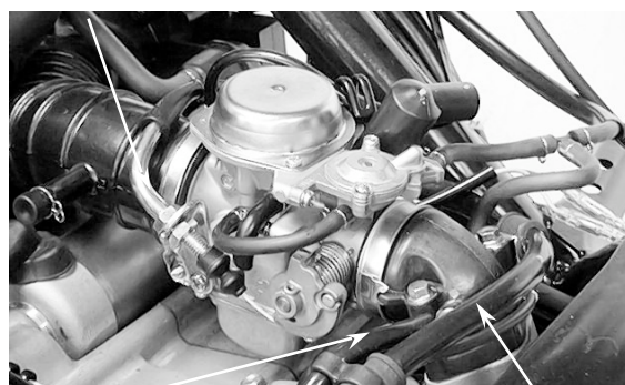
Fuel Pump Vacuum Tube
