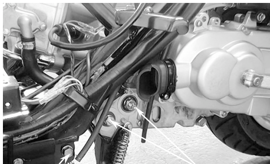
Engine Hanger Bolt Engine Mounting Nuts
