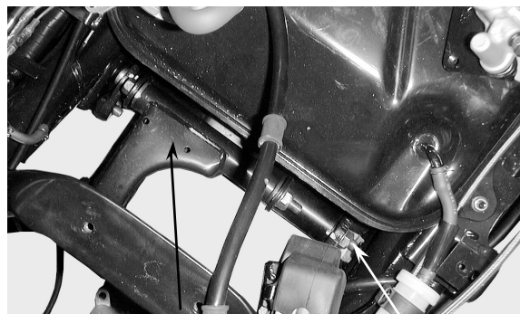
Engine Hanger Bolt
