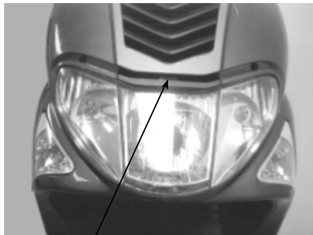
Headlight Aim Adjusting Bolt
