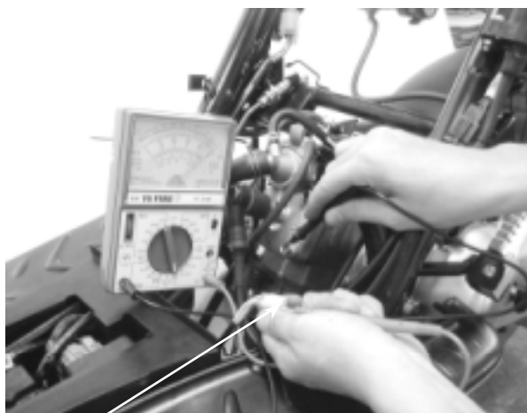
A.C. Generator Connector
