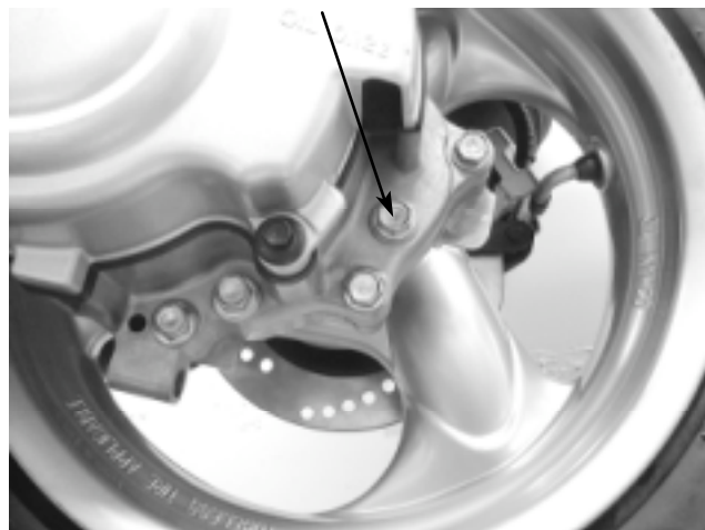
Oil Check Bolt Hole/Oil Filler
