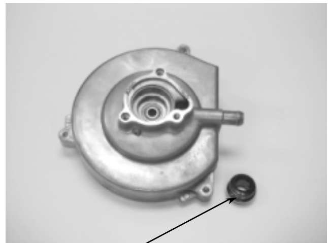
Mechanical Seal
