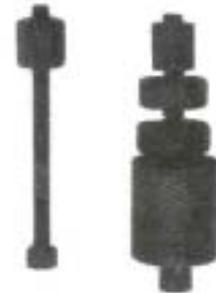
For removing the crankcase suspension bush.
