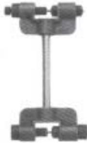
For disassembly the camshaft inner chain.
