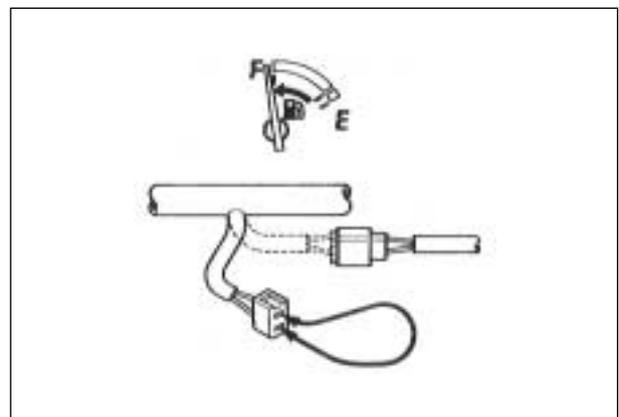
The second test will check the accuracy of the meter in the full and empty positions. Connect a 90 Ω resistor between the Y/B and B/W lead wires. The fuel meter is normal if its pointer indicates the E(empty) position when the specified voltage is applied to the circuit and if its pointer indicates the F(full) position when the resistor is changed to 10 Ω.
