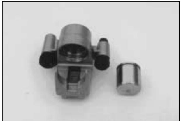
Inspect each rubber part for damage and wear.
