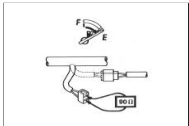
If either one or both indications are abnormal, replace the fuel meter with a new one.
