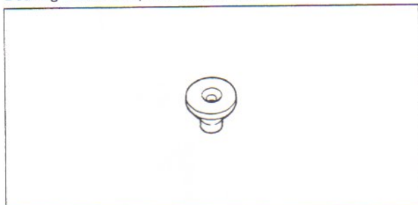
Steering Stem Nut Wrench: 57001-1100
