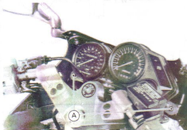
A. Meter Mounting Bolts
