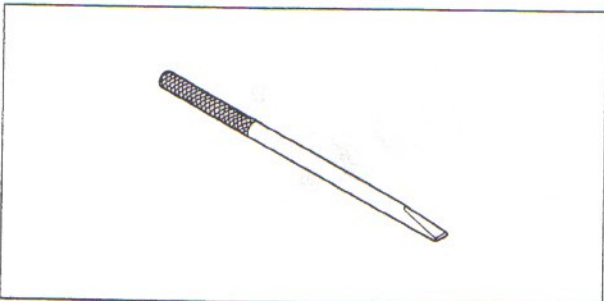
Bearing Remover Shaft: 57001-1265
