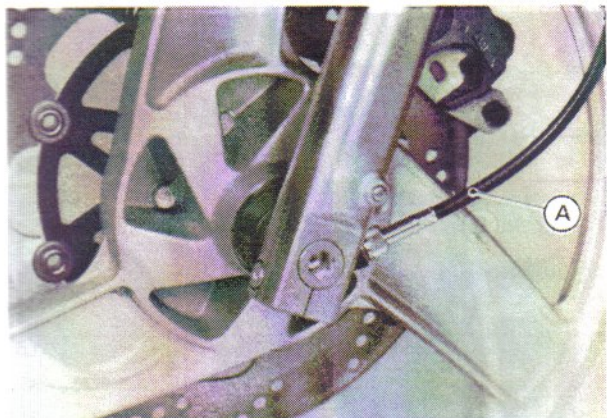
A. Speedometer Cable
