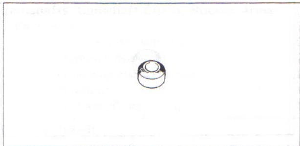
Valve Seat Cutter, 67.5° - \Phi 22 : 57001-1207
