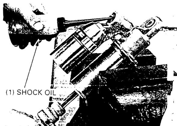
Temporarily charge the reservoir with 7.1 psi (49 kPa, 0.5 kg/cm<sup>2</sup>) of air slowly to inflate the bladder inside.
