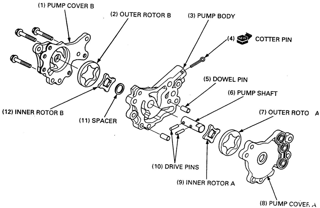
Install the following to the pump body.
