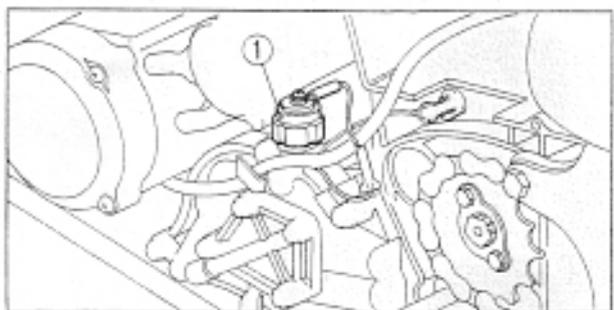
Fig. 5-43 ① Oil pressure control switch
