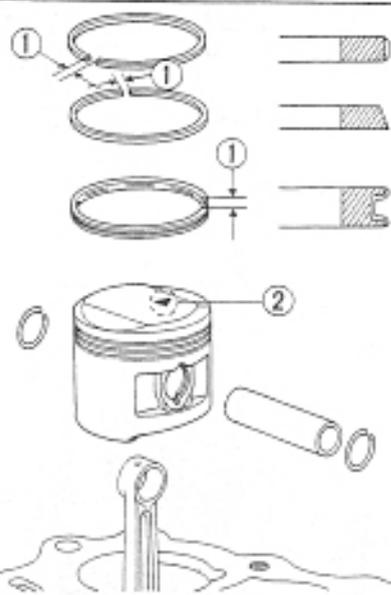
Fig. 3-18 ① Piston ring gap
