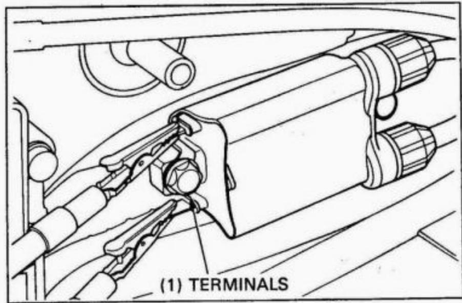
Disconnect the spark plug caps from the spark plug and measure the secondary coil resistance with the spark plug wire at each ignition pair:
