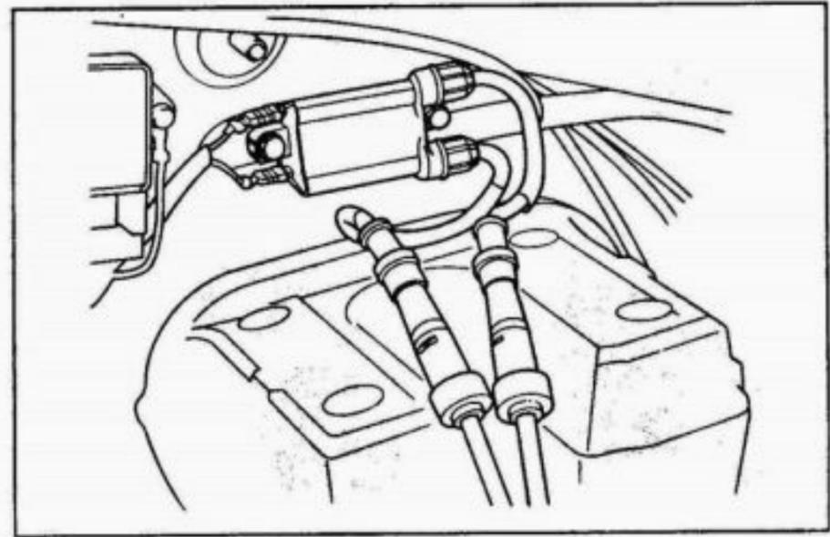
If the resistance is  $\infty$  (open wire), disconnect the spark plug cap and measure the secondary coil resistance as shown.
