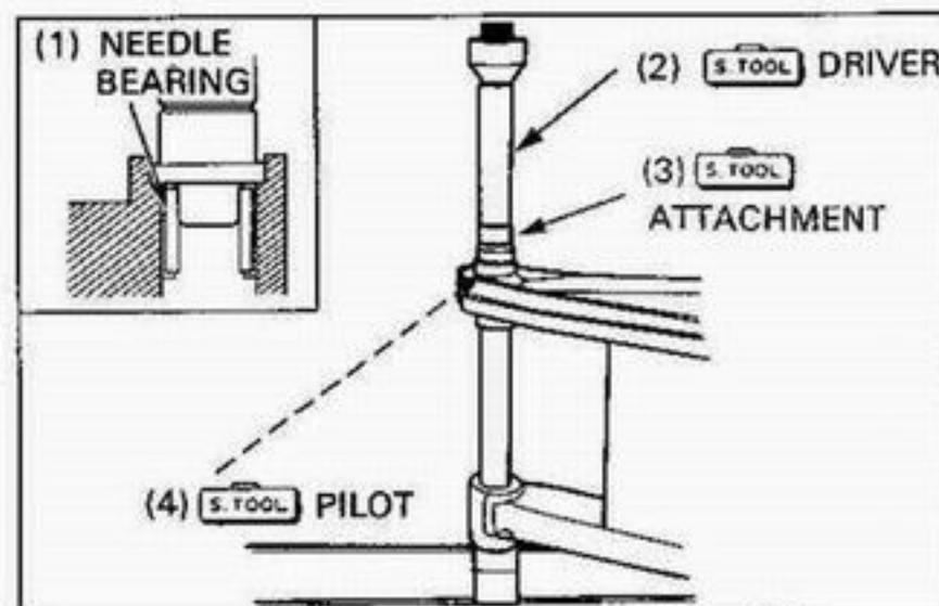
Press the ball bearing in until it bottoms in the swingarm.
