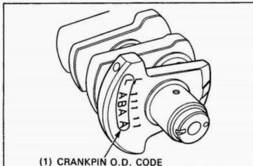
Cross reference the crankpin and rod codes to determine the replacement bearing color code.
