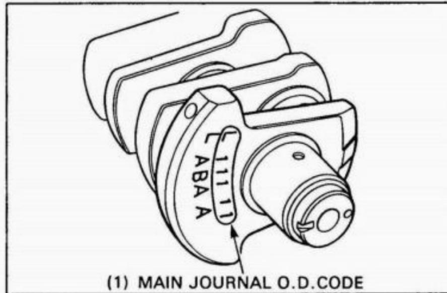
Cross reference the case and journal codes to determine the replacement bearing color code.
