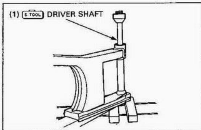
Set the needle bearing remover onto the left pivot bearing (needle bearing) as shown.
