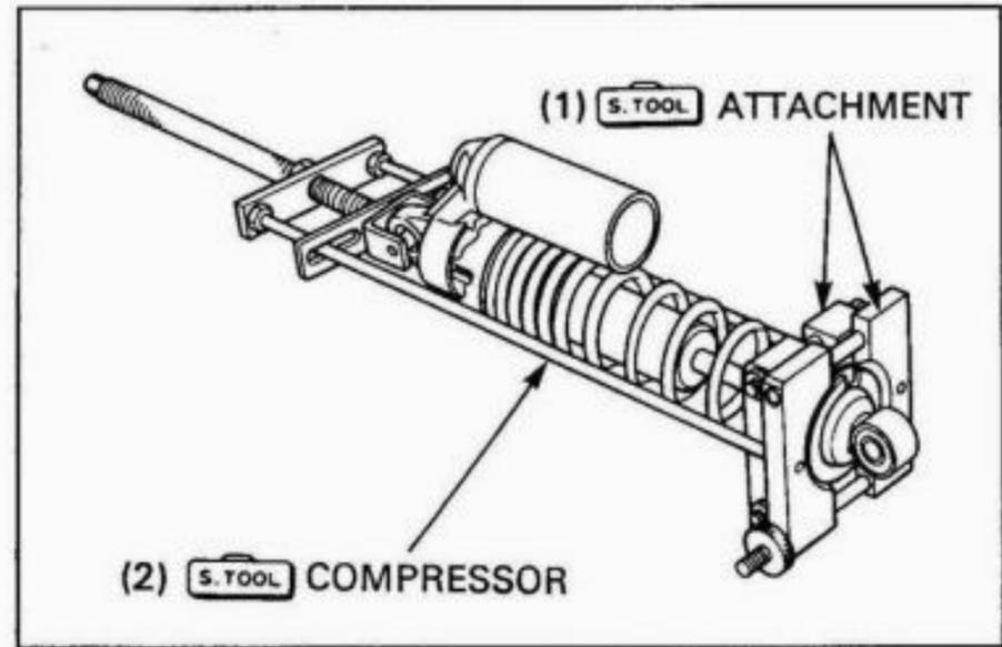
Compress the shock spring and remove the lower seat.
