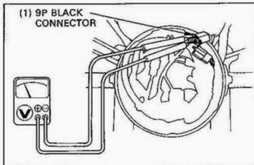
Disconnect the spark unit connector. Check for continuity between the Yellow/Green wire terminals of the 9P mini Black connector and the spark unit connector.
