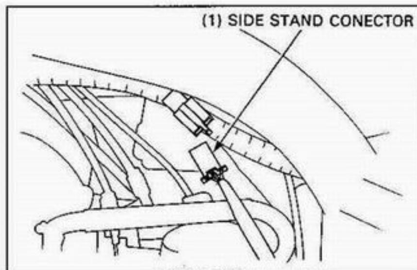
Remove the side stand switch mounting bolt and the side stand switch.
