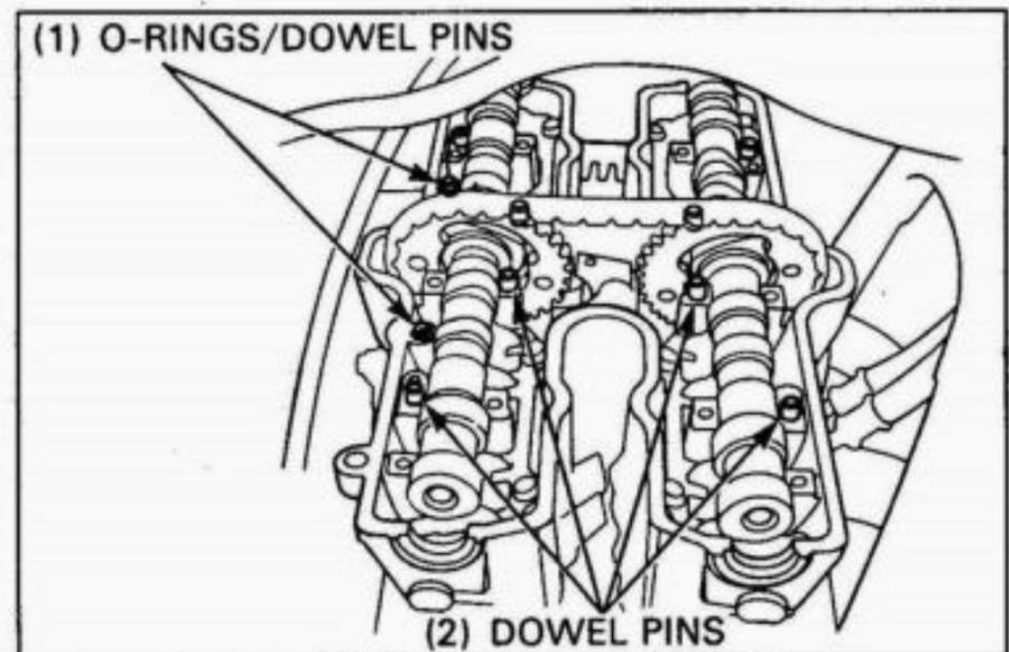
Install each camshaft holder in its original location.
