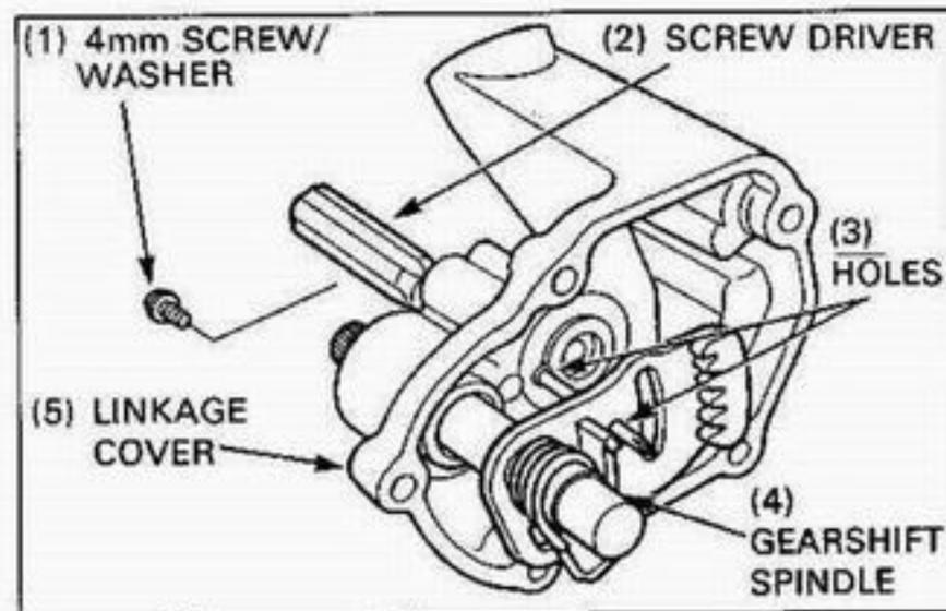
Install the linkage cover/gearshift spindle assembly with the screwdriver through the hole in the shifter.
