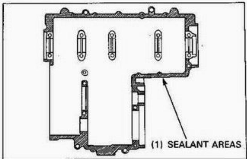
Install the crankcase bolts and sealing washers.
