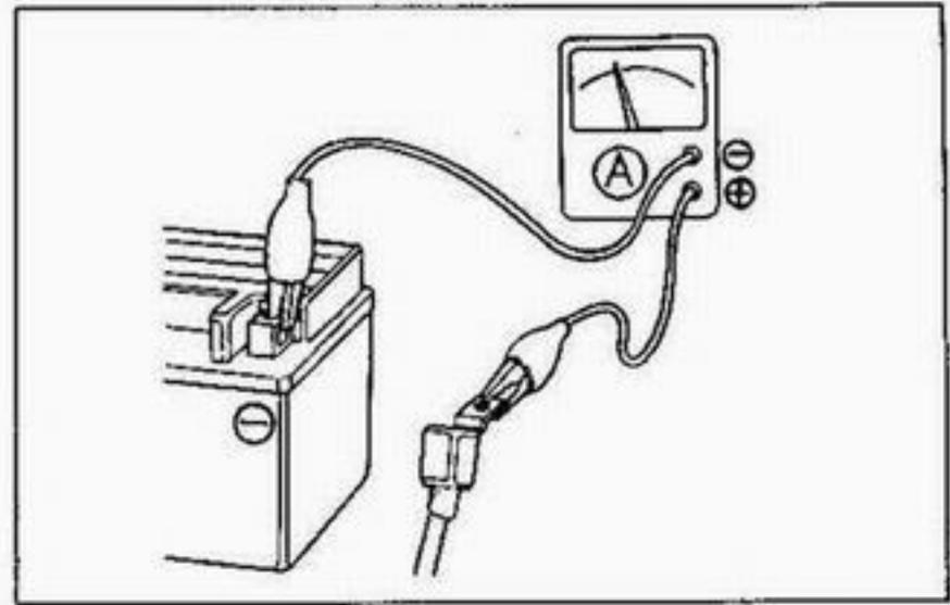
**Specified Current Leakage: 0.01 mA max.**
