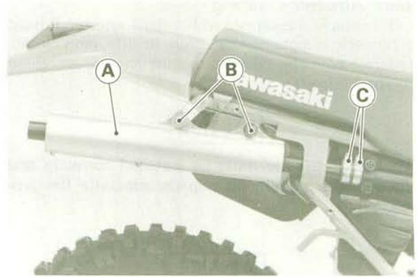
A. Spark Arrester      C. Clamp Screws
