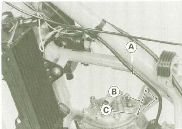
A. Magneto Lead      C. Mounting Bolts
