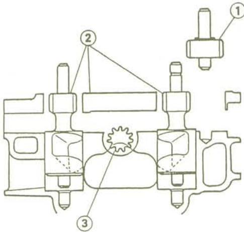
1. Idle Gear      3. Main Exhaust Valve
