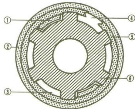
1. Teeth of Toothed Washer      4. Opening of Circlip
