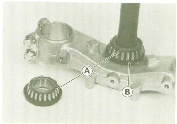
A. Steering Stem (tapered roller) Bearings
