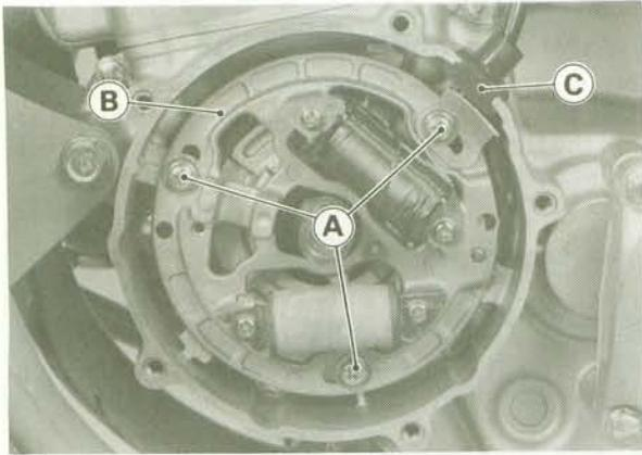
A. Mounting Screws      C. Wiring Grommet
