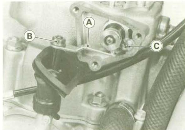
A. Shaft Lever      C. Retaining Screw
