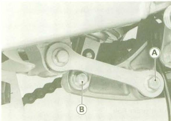
A. Tie-Rod Front Mounting Bolt
