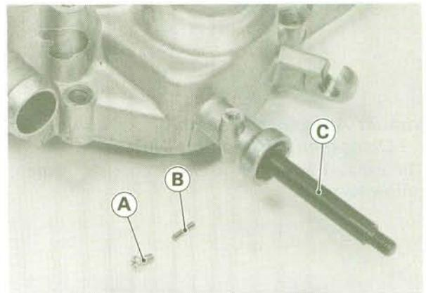
A. Plug Screw                      C. Lever Shaft
