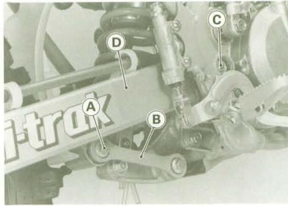
A. Rear Mounting Bolt    C. Swing Arm Pivot Shaft
