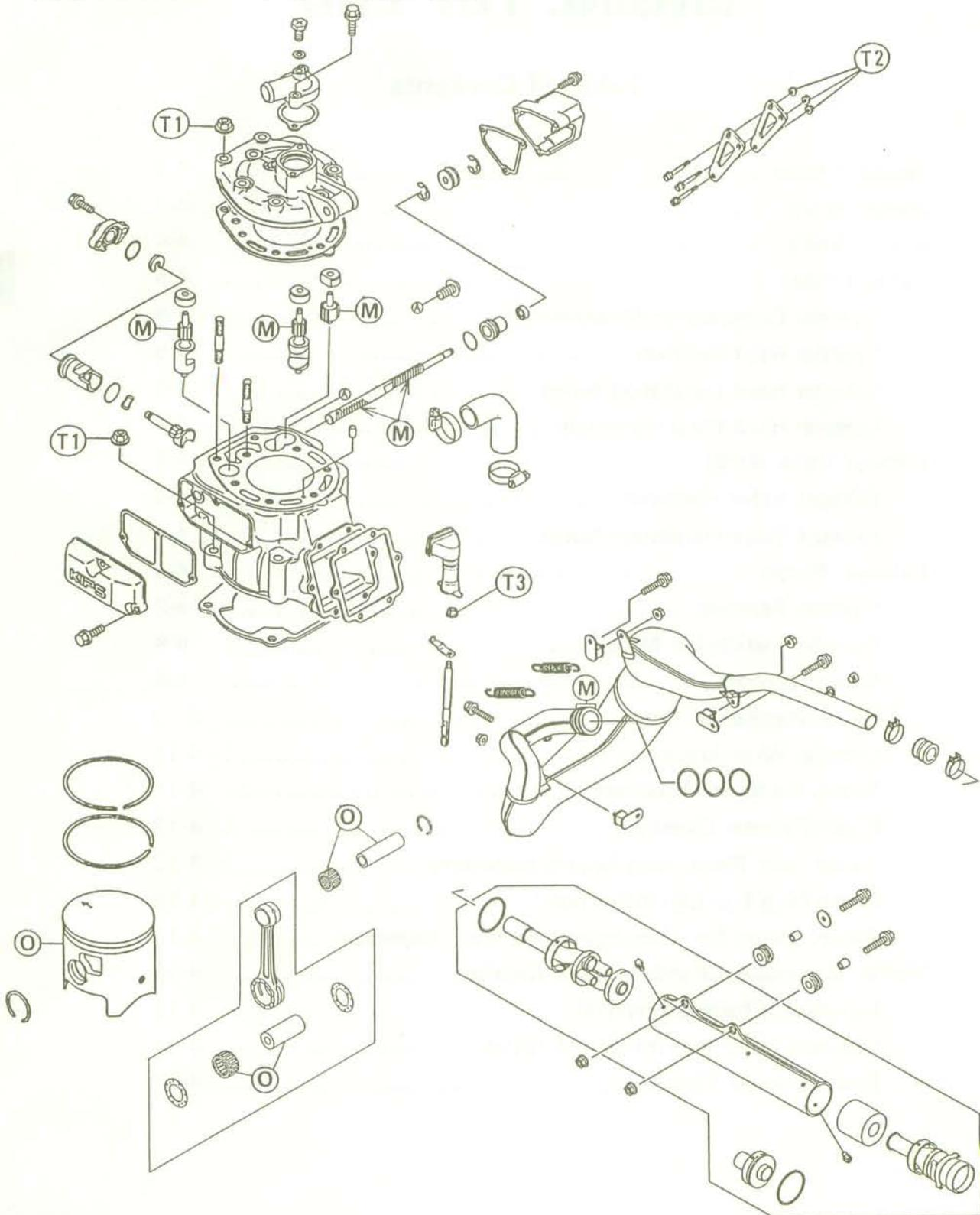
**O:** Apply engine oil to the surface.
