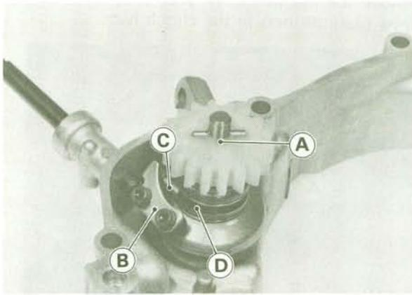
A. Exhaust Advancer Assembly      C. Pin
