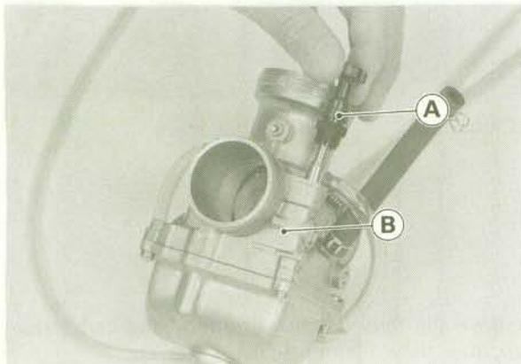
A. Choke Knob/Starter Plunger Assembly
