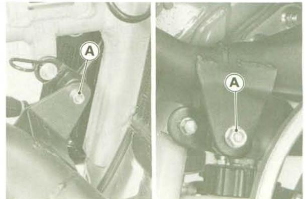
A. Muffler Damper Mounting Nut
