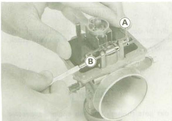
A. Pivot Pin      B. Drive out the pin.
