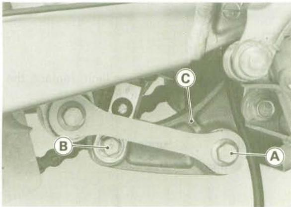
A. Tie-Rod Front Mounting Bolt
