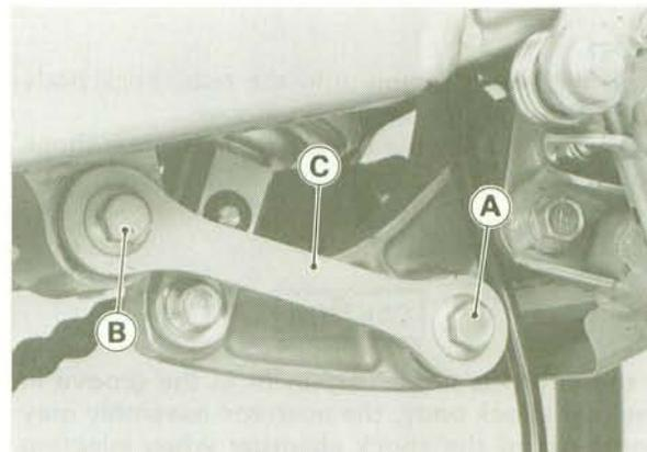
A. Tie-Rod Front Mounting Bolt    C. Tie-Rod
