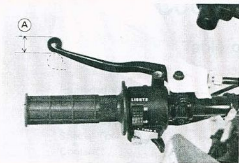
A. Clutch Lever Play (at lever end): 10 – 15 mm
