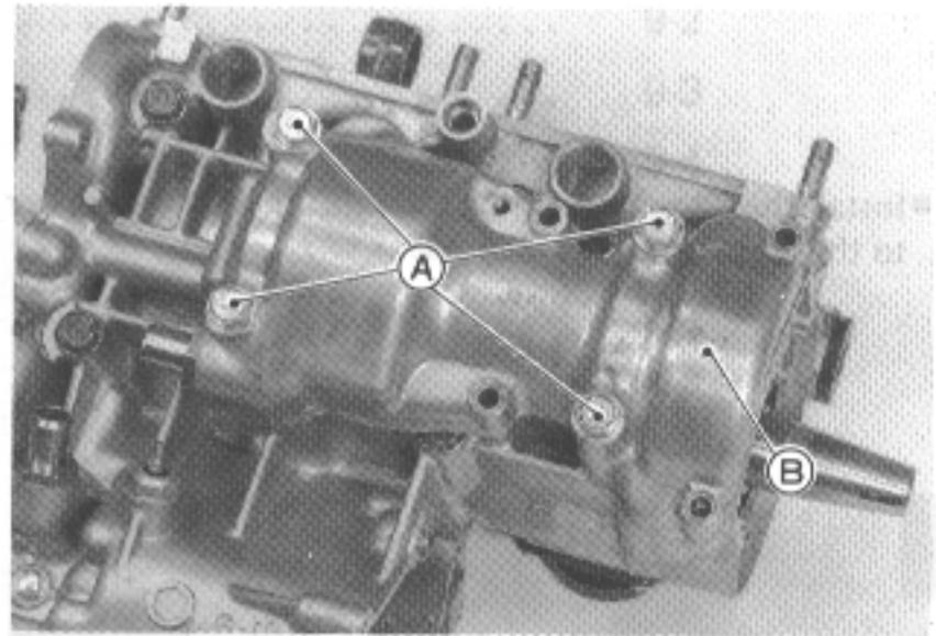
A. Balancer Cover Mounting Bolts (8 mm dia.)
