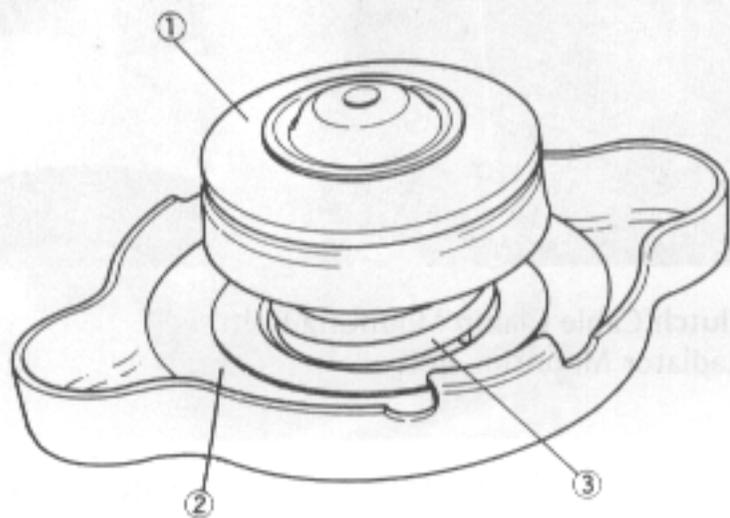
1. Bottom Valve Seal      3. Valve Spring
