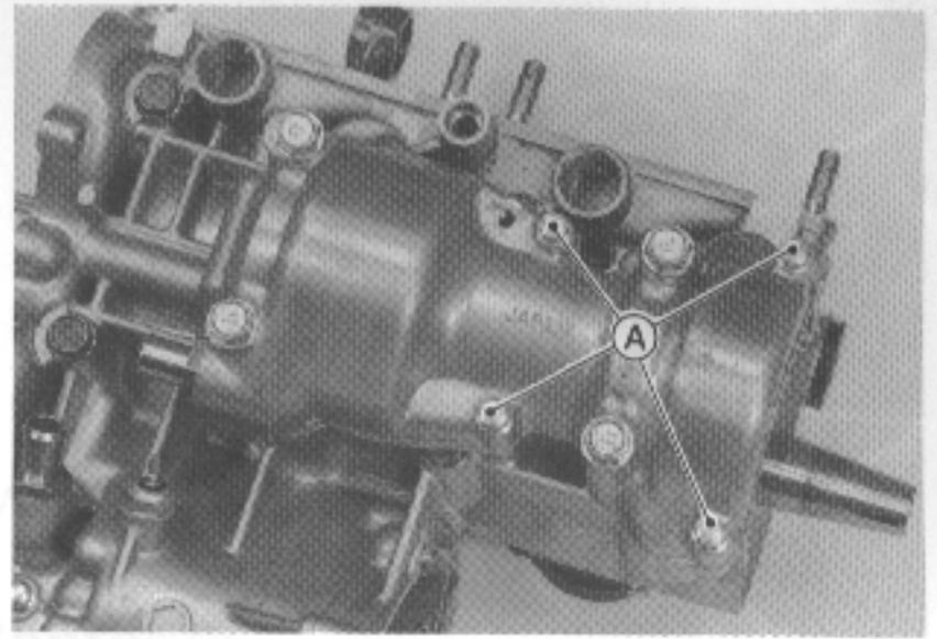
A. Balancer Cover Mounting Bolts (6 mm dia.)
