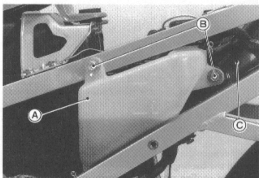
A. Reservoir Tank      C. Rear Fender Front Section
