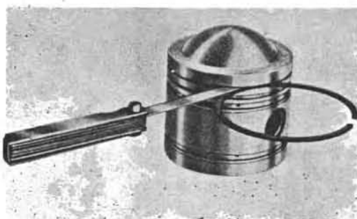
Checking ring-to-piston side clearance
