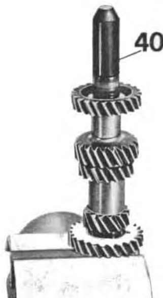
Installing the mainshaft bearing inner race
