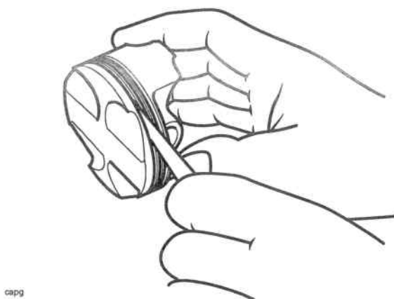
Piston Ring to Ring Groove Clearance Check
