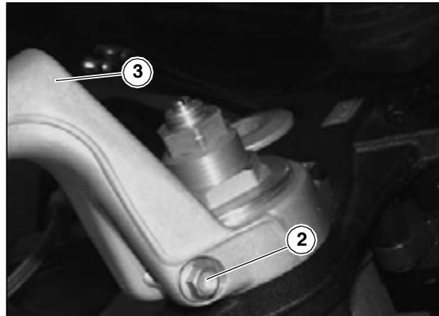
**7.1.19 REMOVING THE RIGHT-HAND HANDLEBAR**
