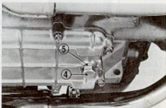
(4) Oil drain plug (5) Sealing washer
