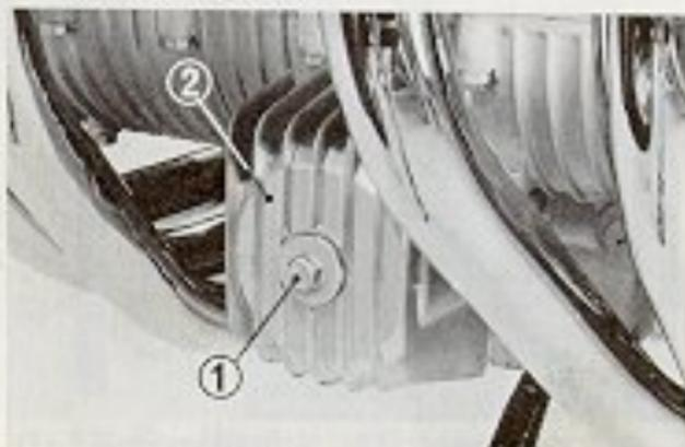
(1) Oil filter lock bolt (2) Oil filter case
