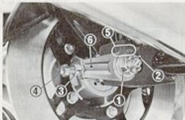
(1) Axle nut (4) Drive chain adjusting bolt
