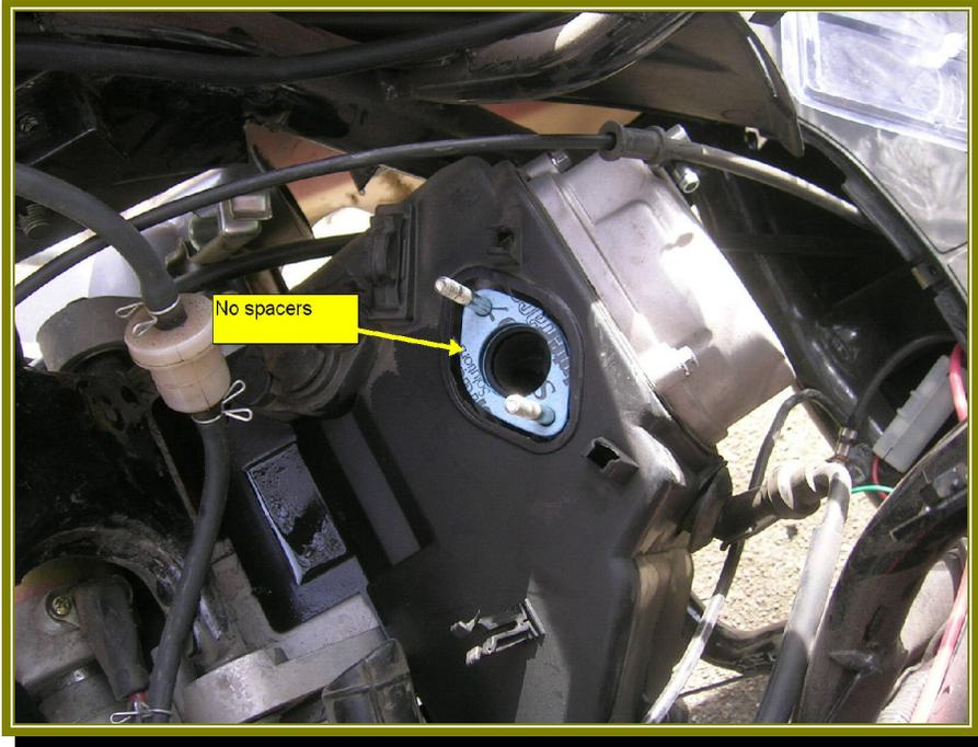
The bottom of the carburetor fits under the crossbar motor mount, not on the top.
