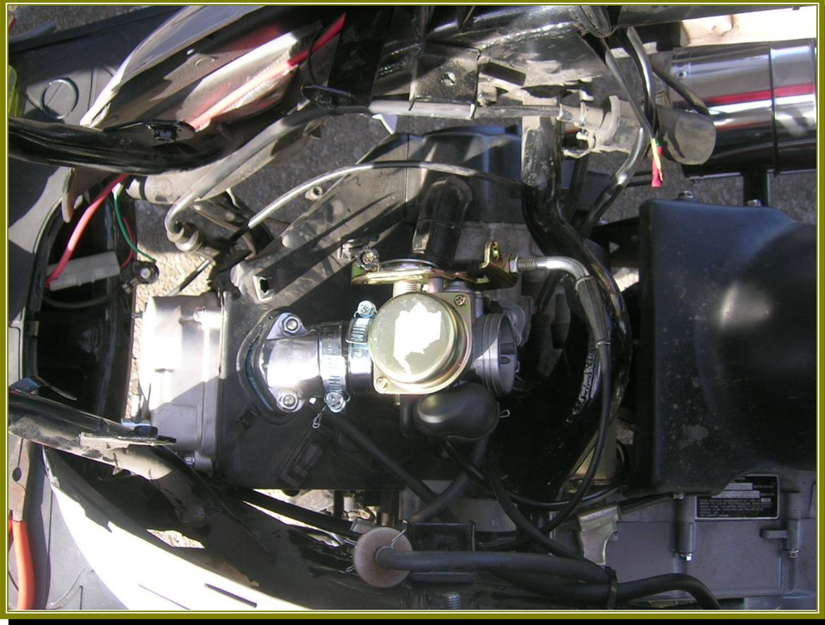
If you find that you can't fit the carburetor into the space in your vehicle, you can modify a stock rubber intake manifold by boring the mouth to proper size to fit the carburetor. Seal with a good quality soft gasket sealant. The stock manifold is shorter, bringing the carburetor closer to the engine.
