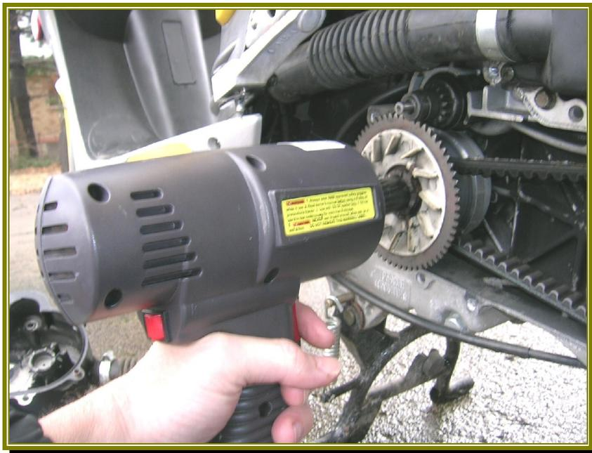
Remove the front fixed pulley.
