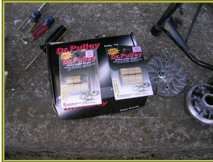
If you are using Dr. Pulley Sliding roller weights, orientation is critical or the variator will not function.
