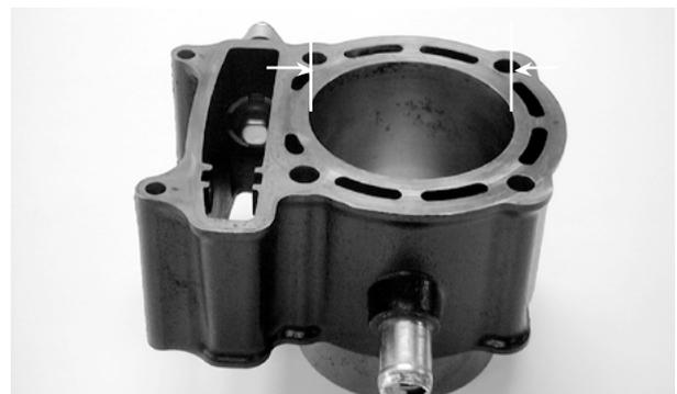
Measure the cylinder-to-piston clearance.
