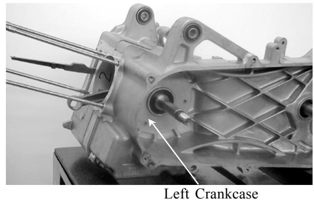
Place the crankcase with the left crankcase down and remove the right crankcase from the left crankcase.
