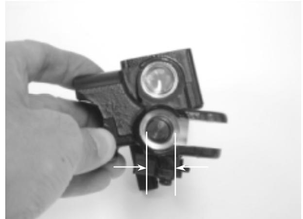
Measure the brake master cylinder piston O.D.
