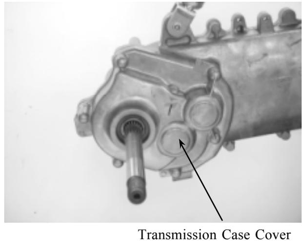
Install and tighten the transmission case cover bolts.
