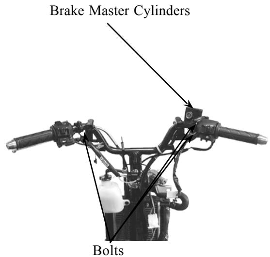
Remove the four screws attaching the right and left handlebar switches.
