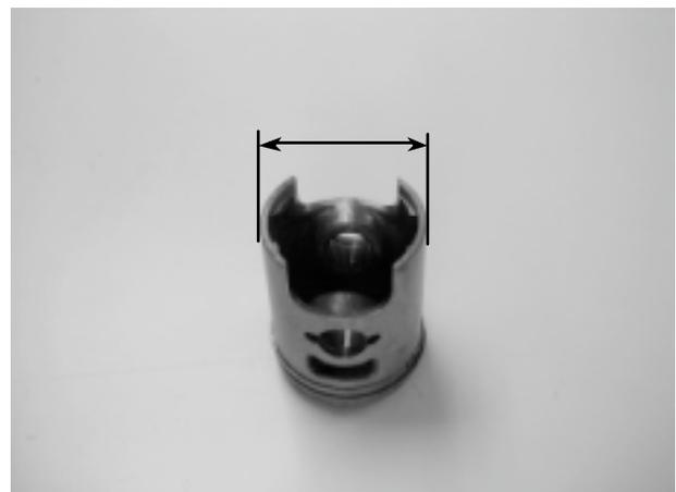
Measure the piston-to-cylinder clearance.
