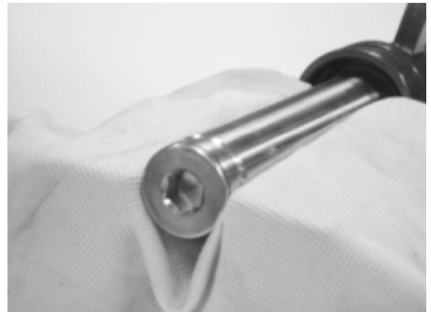
Set the front shock absorber in a vise. Insert the shock absorber tube into the shock absorber and then install the copper washer and tighten the damper rod hex bolt.
