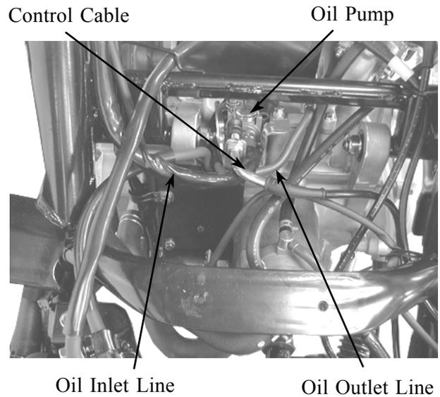
Disconnect the oil pump control cable from the pump body.
