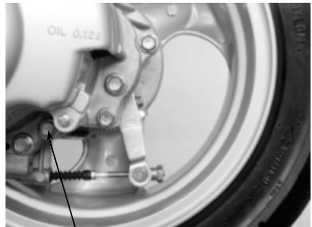
Oil Drain Bolt/Sealing
