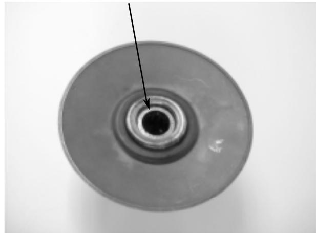
Remove the drive outer bearing out of the driven face.
