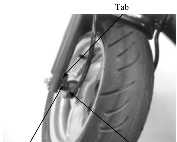
Groove Speedometer Gear Unit
