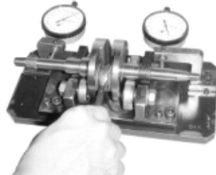
Check the crankshaft bearings for excessive play. The bearings must be replaced if they are noisy or have excessive play.
