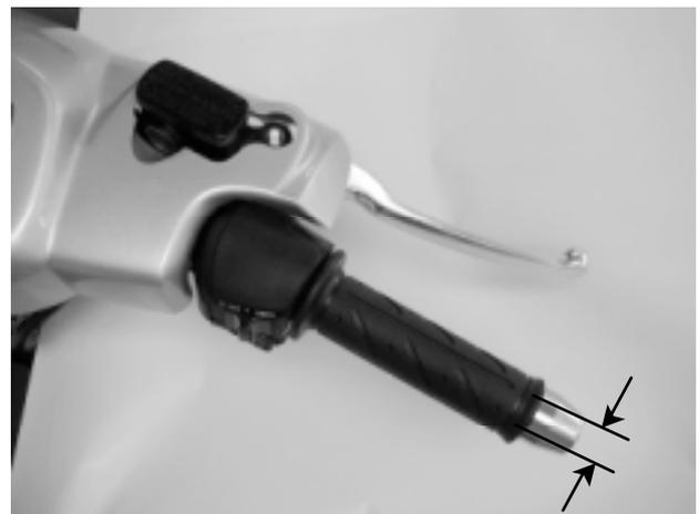
Major adjustment of the throttle grip free play is made with the adjusting nut at the carburetor side. Adjust by loosening the lock nut and turning the adjusting nut.
