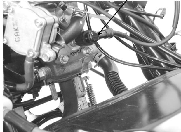
Remove the spark plug cap.
