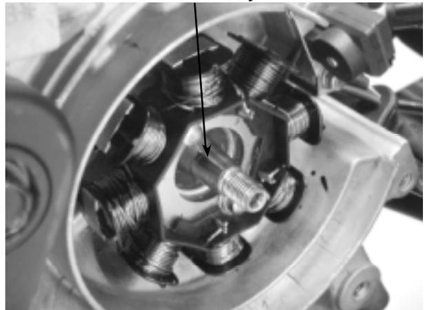
Install the flywheel onto the crankshaft with the flywheel groove aligned with the crankshaft woodruff key.
