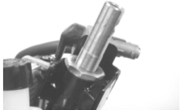
Install the steering stem lock nut and tighten it while holding the top cone race.
