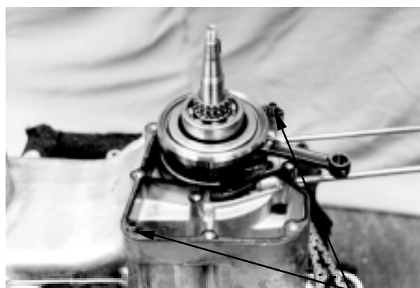
Dowel Pins Crankcase Bolt
