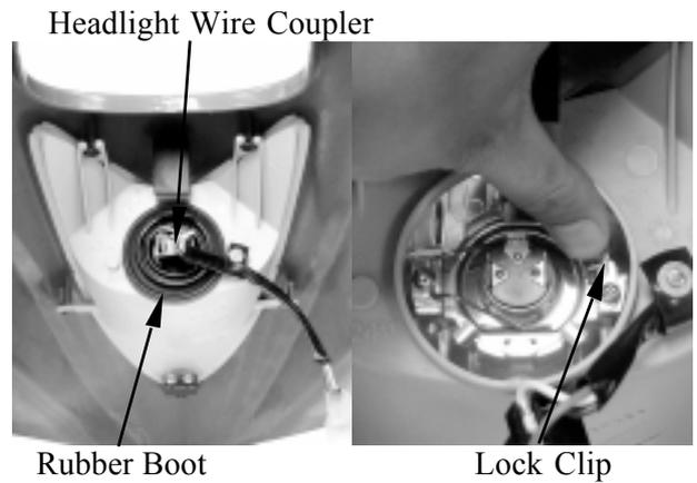
Install the bulb, aligning the bulb socket groove with the bulb tab and set the lock clip.
