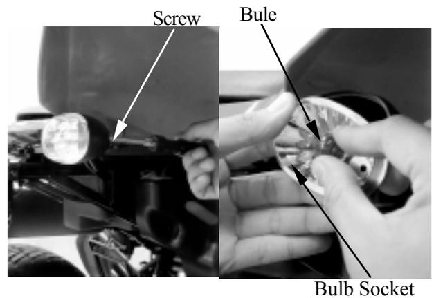
Install the bulb, aligning the bulb socket groove with the bulb tab.
