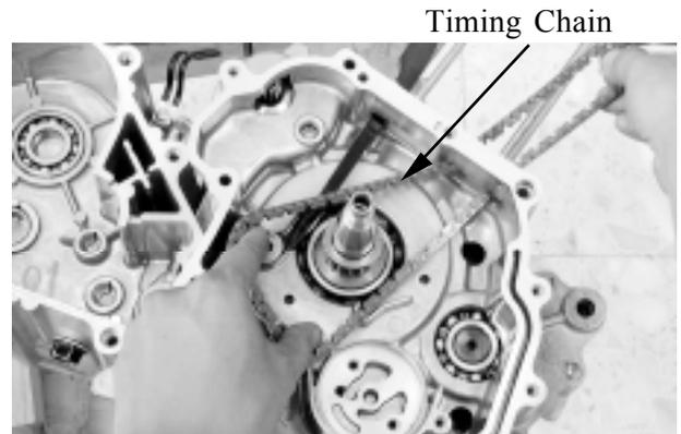
Remove the left and right crankcase attaching bolts.
