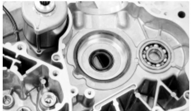
Inspect the balance shaft gear teeth.
