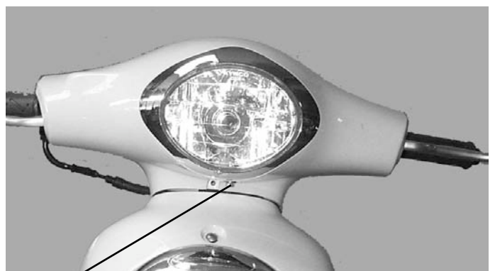
Headlight Adjusting Bolt
