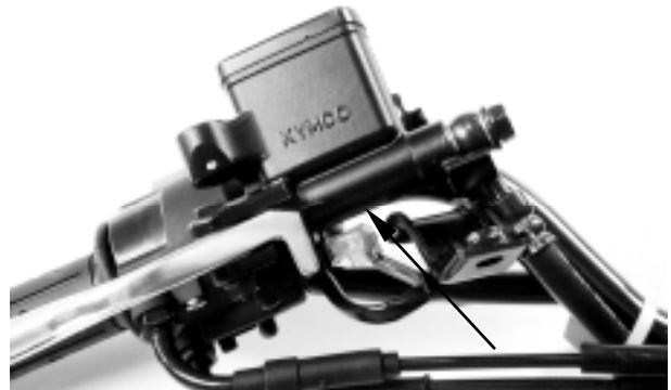
Stop Switch Wire Connector
