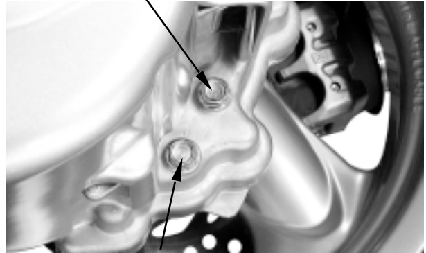
Oil Drain Bolt/Sealing Washer
