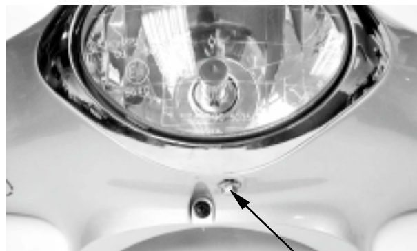
Headlight Aim Adjusting Bolt
