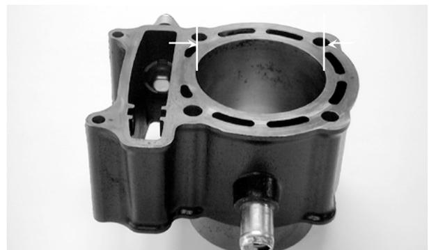
Measure the cylinder-to-piston clearance.
