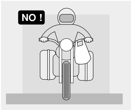
ous objects on the handlebars, mudguards and forks, because the vehicle might respond more slowly in turns and its manoeuvrability could be unavoidably impaired.
